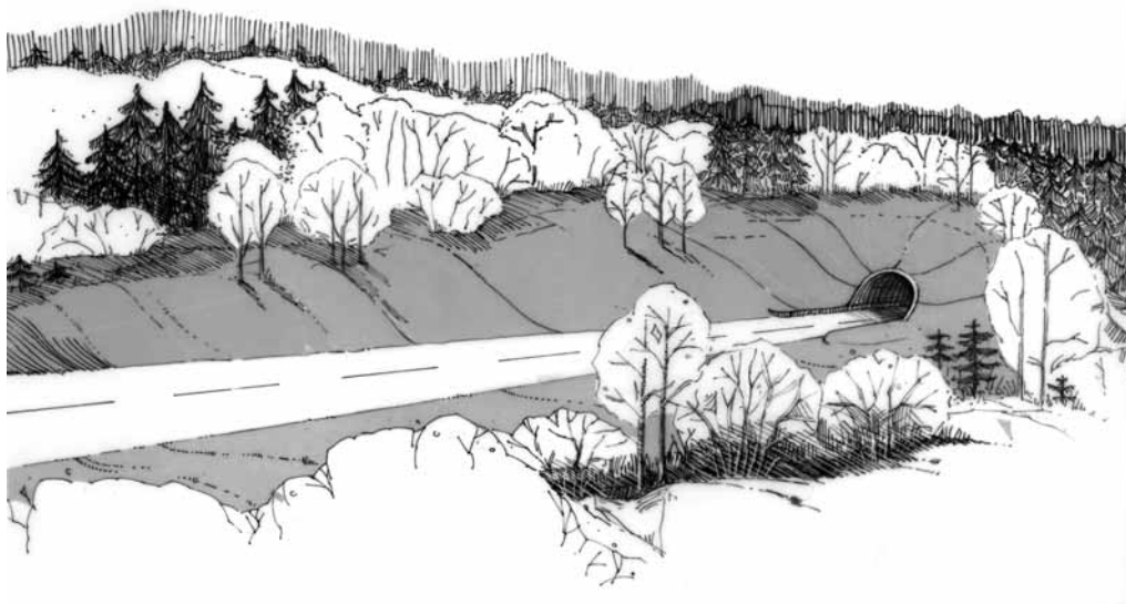
Figure 5.4 Approach zone in an area with slight gradient. In order to avoid the impression of entering a shaft at the tunnel entrance, the landscape has been comprehensively planned. Illus. Ingeborg Langeland Degnes.
