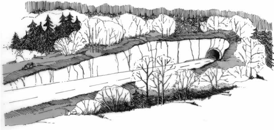
Figure 5.3 Approach zone in an area with slight gradient. The cutting is long and deep and does not give a clear impression of approaching a tunnel. Illus. Ingeborg Langeland Degnes.
