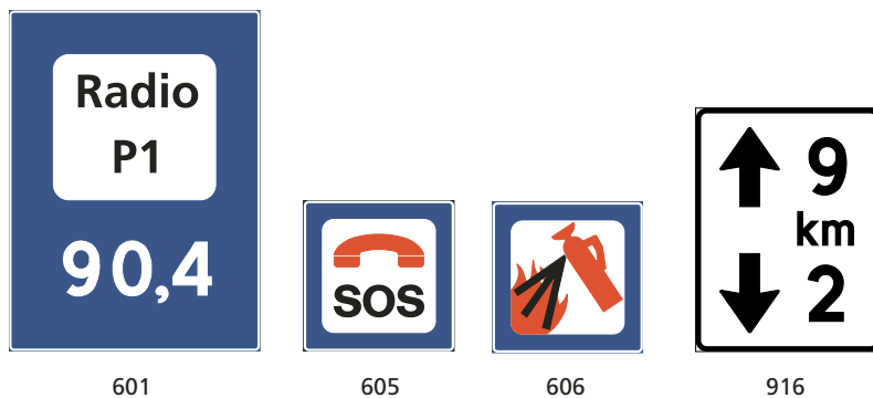
Figure 4.24 Signs used in the tunnel
