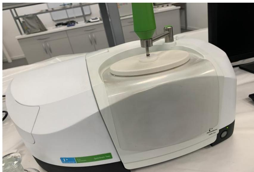
*Slika 15. PerkinElmer Spectrum Two FT-IR spektrometar*
