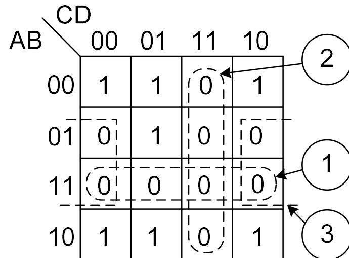
$$F = (\bar{A} + \bar{B}) \cdot (\bar{C} + \bar{D}) \cdot (\bar{B} + D)$$
