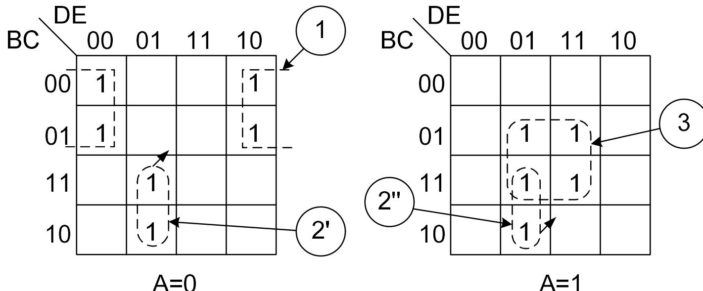
$$F = \overline{A}\overline{B}\overline{E} + B\overline{D}E + ACE$$
