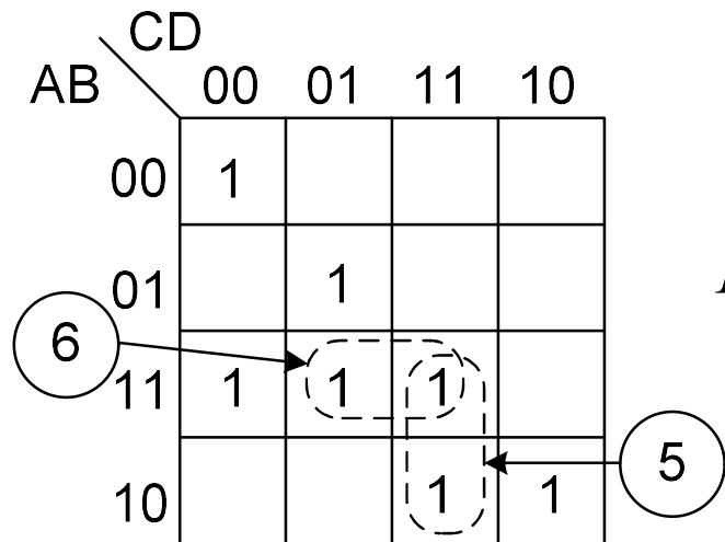
$$F = \overline{A}\overline{B}\overline{C}\overline{D} + B\overline{C}D + A\overline{B}\overline{C} + A\overline{B}C + \begin{cases} ACD \\ ili \\ ABD \end{cases}$$
