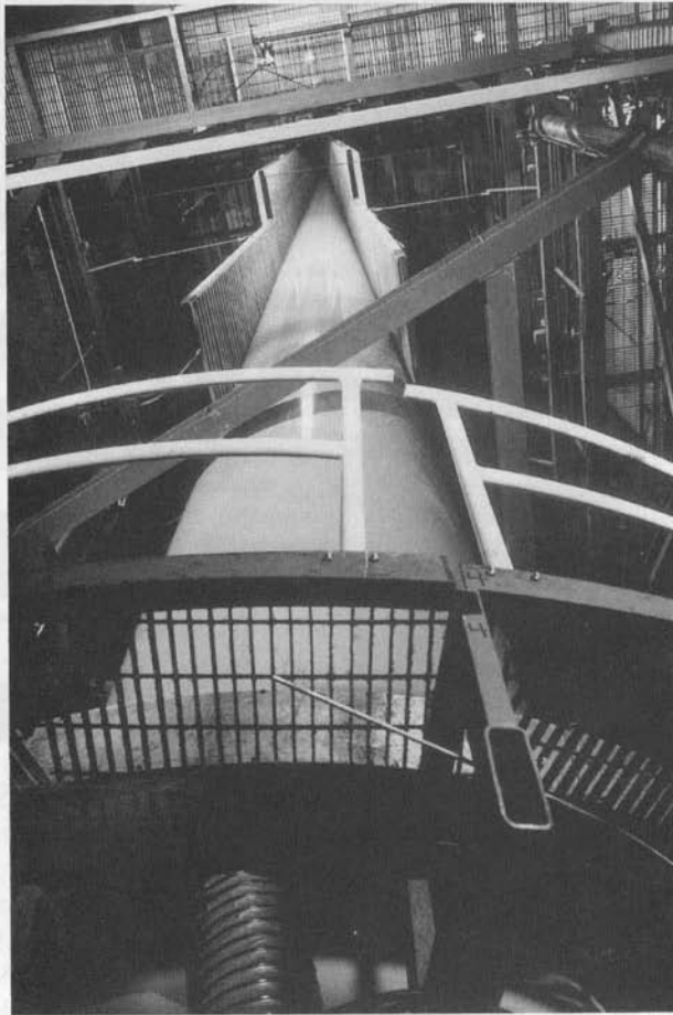
Figure 1.22 Processing of geomembranes by blown sheet extrusion. (Compliments of GSE Lining Technology, Inc.)
