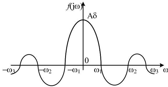
$$F(j\omega) = \frac{2A}{\omega} \sin \frac{\omega\delta}{2} = 2A \frac{\delta}{2} \frac{\sin \frac{\omega\delta}{2}}{\frac{\omega\delta}{2}} = A\delta \frac{\sin \frac{\omega\delta}{2}}{\frac{\omega\delta}{2}}$$
