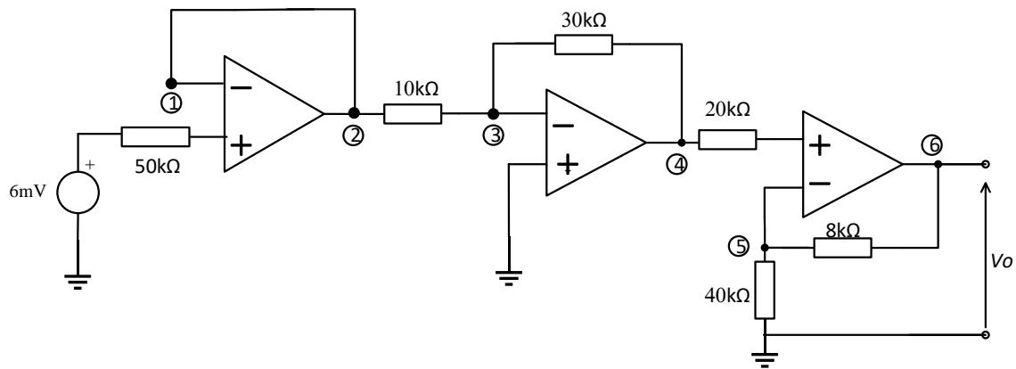
$$V_1 = V_2 = 6mV$$
