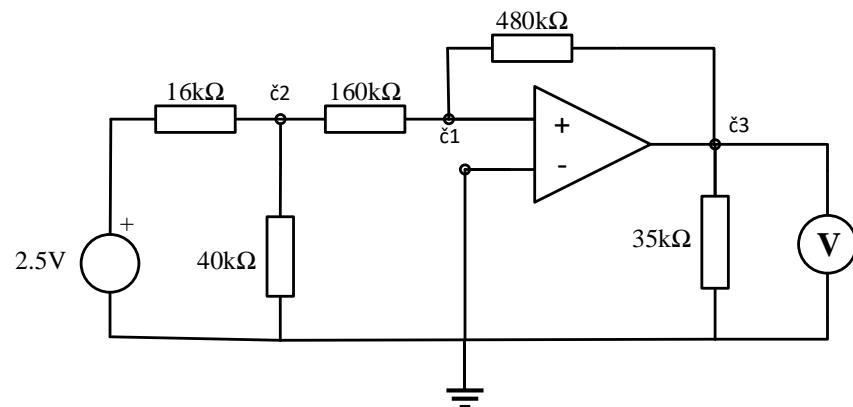
$$V_+ = V_- = V_i = 0$$
