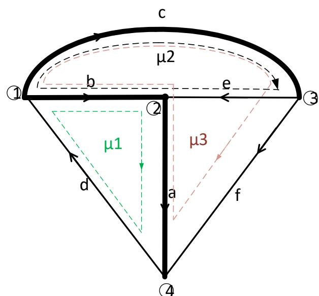
$$B_f = \begin{bmatrix} a & b & c & d & e & f \\ 1 & 1 & 0 & 1 & 0 & 0 \\ 0 & -1 & 1 & 0 & 1 & 0 \\ \sim & \sim & \sim & \sim & \sim & \sim \\ -1 & -1 & 1 & 0 & 0 & 1 \end{bmatrix}$$
