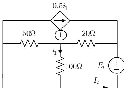
$$\left( \frac{1}{50} + \frac{1}{20} + \frac{1}{100} \right) v_1 - \frac{1}{20} E_t = 0 \Rightarrow E_t = 1.6v_1 = 160i_1$$
