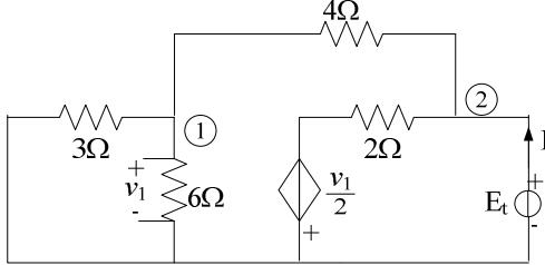
$$\left(\frac{1}{3} + \frac{1}{6} + \frac{1}{4}\right)v_1 - \frac{1}{4}v_2 = 0$$
