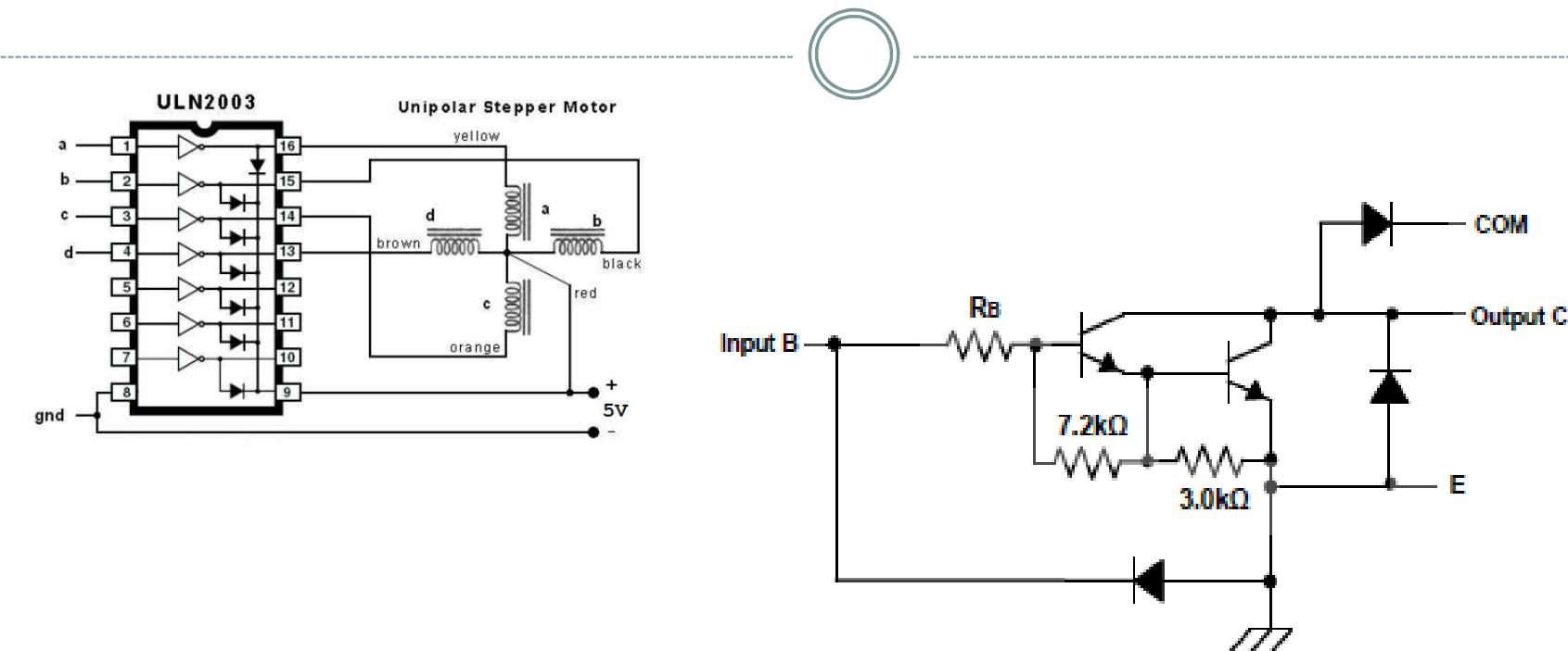
ULN2003A:  $R_B = 2\text{k}\Omega$
