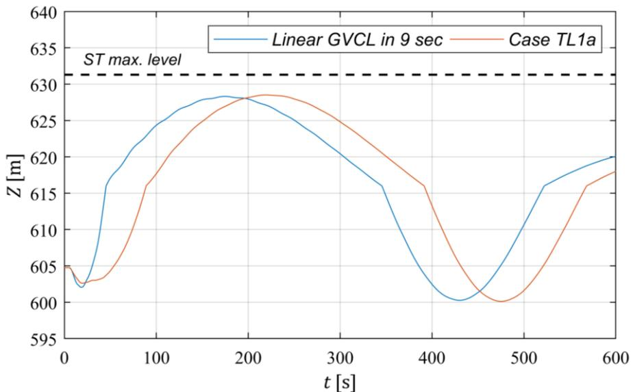
Fig. 4 STWL for linear in 9 sec and tri-linear TL1a GVCL
