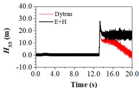
**Figure 2.** Comparison of heads at the position 3/3 measured by Dytran piezoelectric and E+H strain-gauge pressure transducers: pipeline filling [5].
