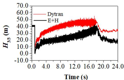
**Figure 4.** Comparison of heads at the position 3/3 measured by Dytran piezoelectric and E+H strain-gauge pressure transducers: pipeline emptying [5].
