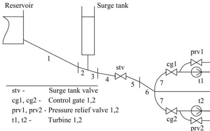
Fig. 1 Hydropower plant Pirot - scheme[2]
