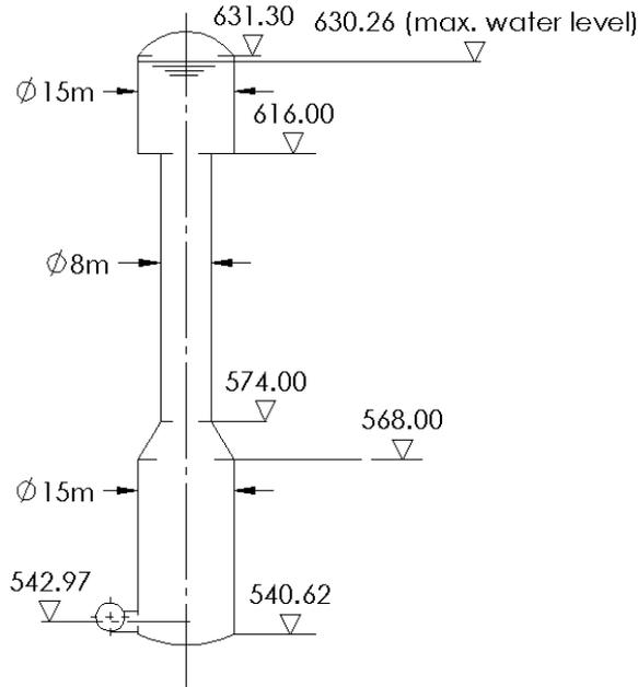
Fig. 2 Hydropower plant Pirot – surge tank [4]
