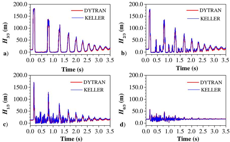
Fig. 3 Comparison of heads at the valve units (positions  $p_{0/3}$ ,  $p_{1/3}$ ,  $p_{2/3}$  and  $p_{3/3}$ )
