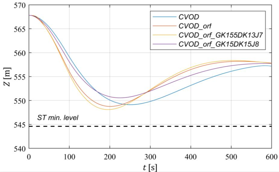
Fig. 6 STWL for 90 sec simultaneous start for different surge tank types
