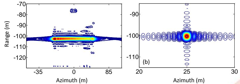
MT3 contour image ((a): range focused image after range walk correction; (b): final focused image).
