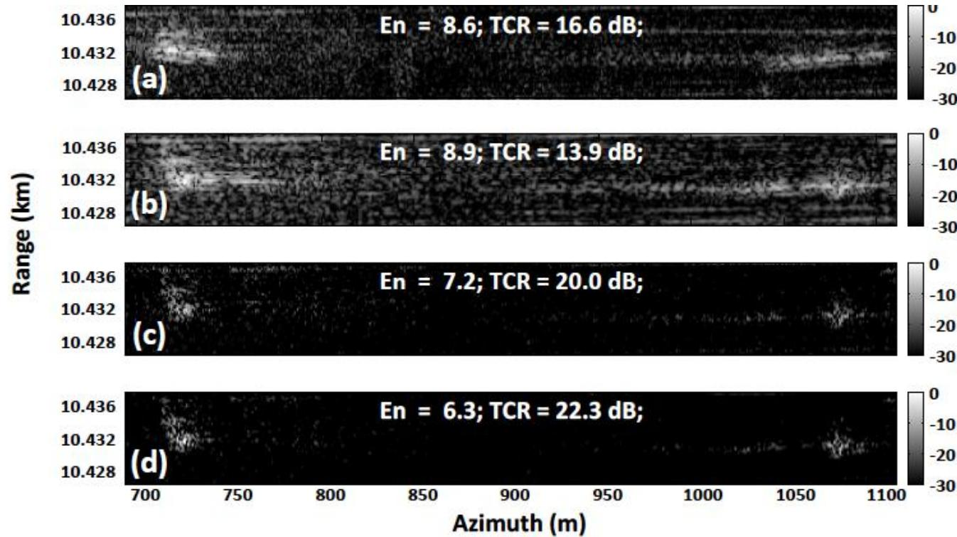
Real data processing results ((a): SAR image with 2 moving targets formed by FFT with full data sample; (b)-(d): SAR moving target image by MF, CS and para-BCS, respectively, 1/2 data undersampling ratio.
