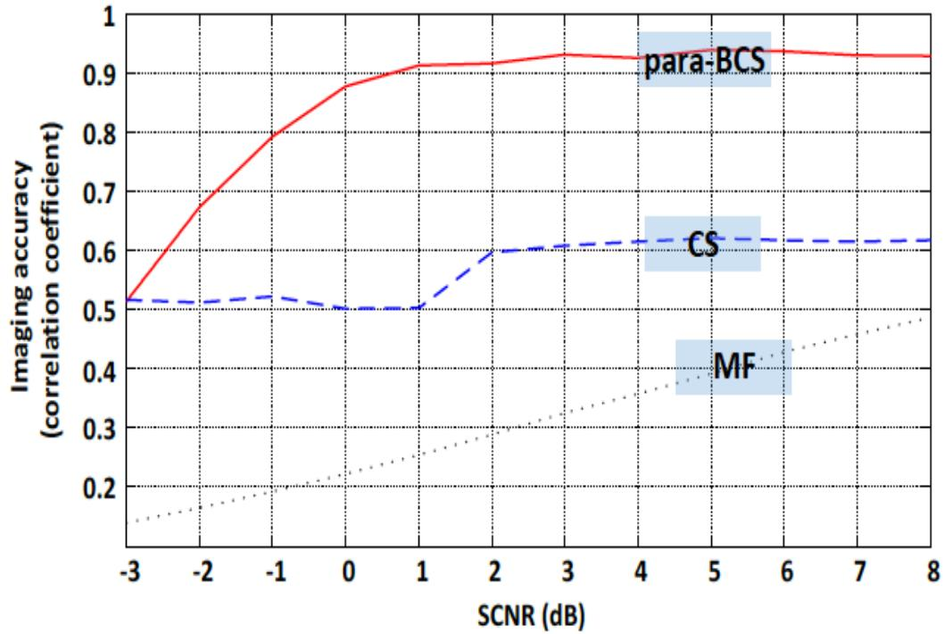
Imaging accuracy comparison (1/2 under sampling data ratio and multiplicative phase error)
