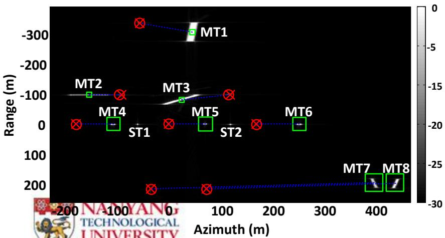
SAR moving target imaging results. Circle: moving target ground truth; Square: displaced and defocused moving target; Cross: geolocated and refocused moving target by the proposed algorithm.
