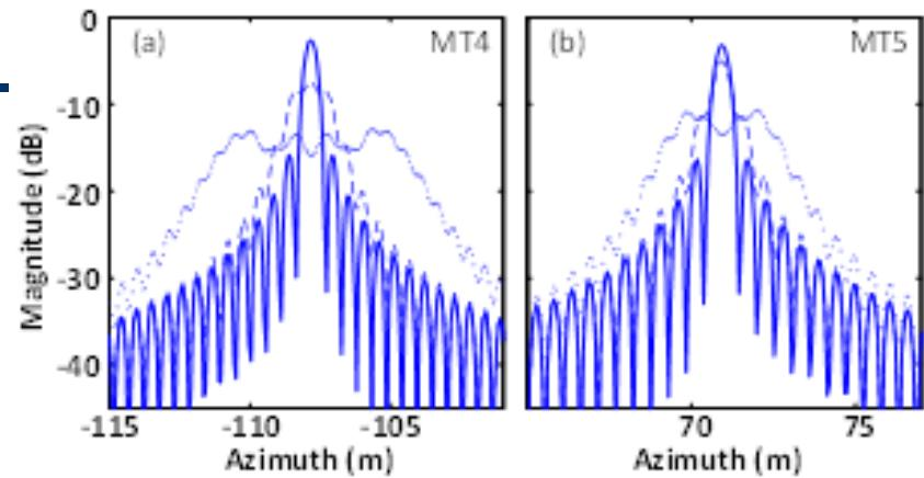
Azimuth responses of defocused and refocused (a) MT4, (b) MT5 (dotted line: defocused target response; dashed line: refocused target response based on FrFT representation; solid line: refocused target response based on LVD representation).
