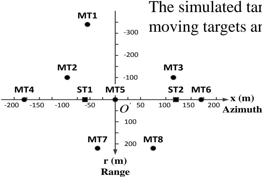
The simulated target ground truth for 8 moving targets and 2 stationary targets.
