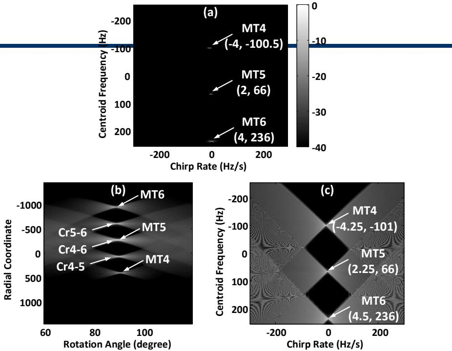
TFR for MT4-MT6: (a) LVD, (b) RWT and (c) FrFT, (RWT is with rotational angle searching step  $0.1^\circ$ , and FrFT is with rotational order searching step 0.0002)
