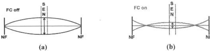
Figure 9. Schematic of level variation mechanism: (a) FC off, (b) FC on
