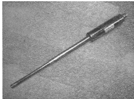
Figure 1: Ultrasonic sensor with stainless steel wave-guide
