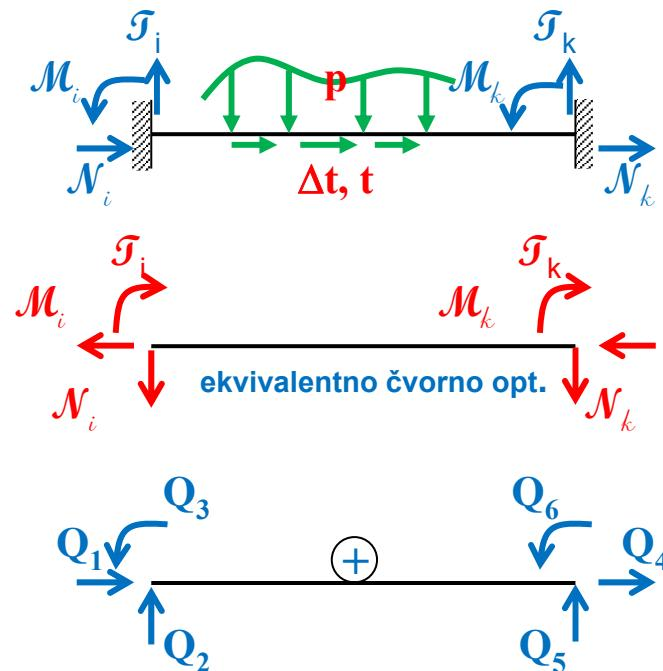
$$\begin{bmatrix} Q_1 \\ Q_2 \\ Q_3 \\ Q_4 \\ Q_5 \\ Q_6 \end{bmatrix} = - \begin{bmatrix} \mathcal{N}_i \\ \mathcal{T}_i \\ \mathcal{M}_i \\ \mathcal{N}_k \\ \mathcal{T}_k \\ \mathcal{M}_k \end{bmatrix}$$
