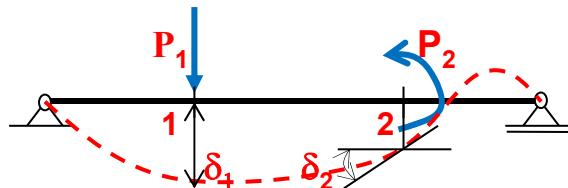
$$\begin{bmatrix} \delta_1 \\ \delta_2 \end{bmatrix} = \begin{bmatrix} f_{11} & f_{12} \\ f_{21} & f_{22} \end{bmatrix} \begin{bmatrix} P_1 \\ P_2 \end{bmatrix}$$
