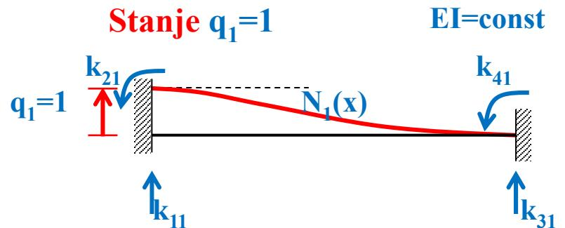
$$\begin{bmatrix} R_1 \\ R_2 \\ R_3 \\ R_4 \end{bmatrix} = \begin{bmatrix} k_{11} & k_{12} & k_{13} & k_{14} \\ k_{21} & k_{22} & k_{23} & k_{24} \\ k_{31} & k_{32} & k_{33} & k_{34} \\ k_{41} & k_{42} & k_{43} & k_{44} \end{bmatrix} \begin{bmatrix} 1 \\ 0 \\ 0 \\ 0 \end{bmatrix} = \begin{bmatrix} k_{11} \\ k_{21} \\ k_{31} \\ k_{41} \end{bmatrix}$$
