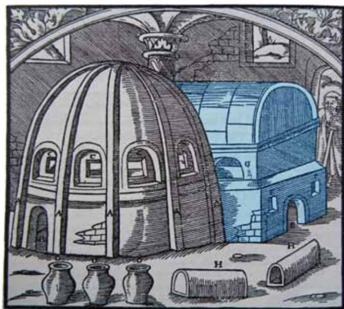
A—ARCIES OF THE SECOND FURNACE. B—MOUTH OF THE LOWER CHAMBER. C—WINDOWS OF THE UPPER CHAMBER. D—BIG-BELLIED POTS. E—MOUTH OF THE THIRD FURNACE. F—RECESSES FOR THE RECEPTACLES. G—OPENINGS IN THE UPPER CHAMBER. H—OBLONG RECEPTACLES.
