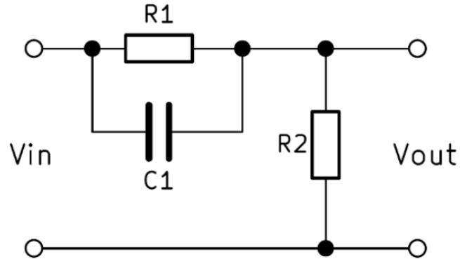
$$A(s) = \frac{R_2}{R_1 + R_2} \frac{1 + sC_1 R_1}{1 + sC_1 (R_1 \parallel R_2)}$$
