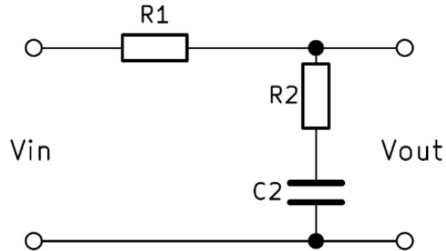
$$A(s) = \frac{1 + sC_2R_2}{1 + sC_2(R_1 \parallel R_2)}$$
