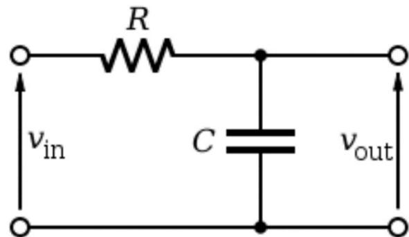
$$A(s) = \frac{V_{out}(s)}{V_{in}(s)} = \frac{\frac{1}{sC}}{R + \frac{1}{sC}}$$
