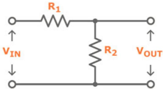
$$V_{out} = \frac{R_2}{R_1 + R_2} V_{ul}$$
