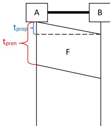
$$t_{\text{prop}} = \frac{l}{v} = \frac{250\text{m}}{2,5 \cdot 10^8 \text{ m/s}} = 1\mu\text{s}$$
