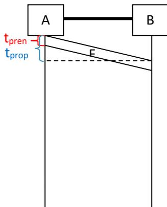
$$t_{\text{prop}} = \frac{l}{v} = \frac{250\text{m}}{2,5 \cdot 10^8 \text{ m/s}} = 1\mu\text{s}$$
