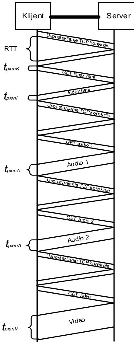
$$t_{uk} = 8RTT + t_{prenI} + 2t_{prenA} + t_{prenV} + 12t_{prenK} = 16t_{prop} + \frac{L_I}{R} + 2\frac{L_A}{R} + \frac{L_V}{R} + 12\frac{L_K}{R}$$
