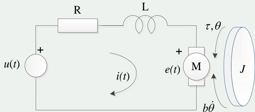
$$\frac{d}{dt} \begin{bmatrix} \theta \\ \dot{\theta} \\ i \end{bmatrix} = \begin{bmatrix} 0 & 1 & 0 \\ 0 & -b/J & k/J \\ 0 & -k/L & -R/L \end{bmatrix} \begin{bmatrix} \theta \\ \dot{\theta} \\ i \end{bmatrix} + \begin{bmatrix} 0 \\ 0 \\ 1/L \end{bmatrix} u$$
