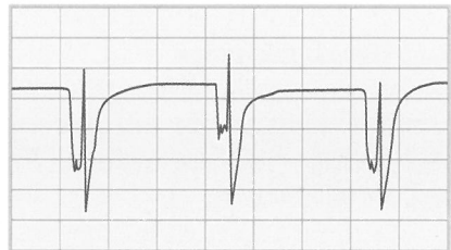
Fig. 17: with SikaPump®: continuous pumping pressure
