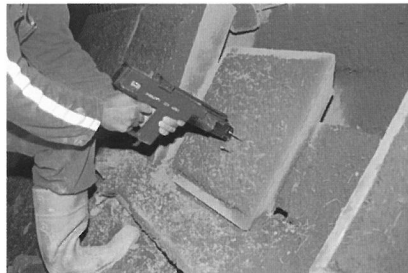
Fig. 36: very early strength from 1 to 15 N/mm 2 with bolt firing method
