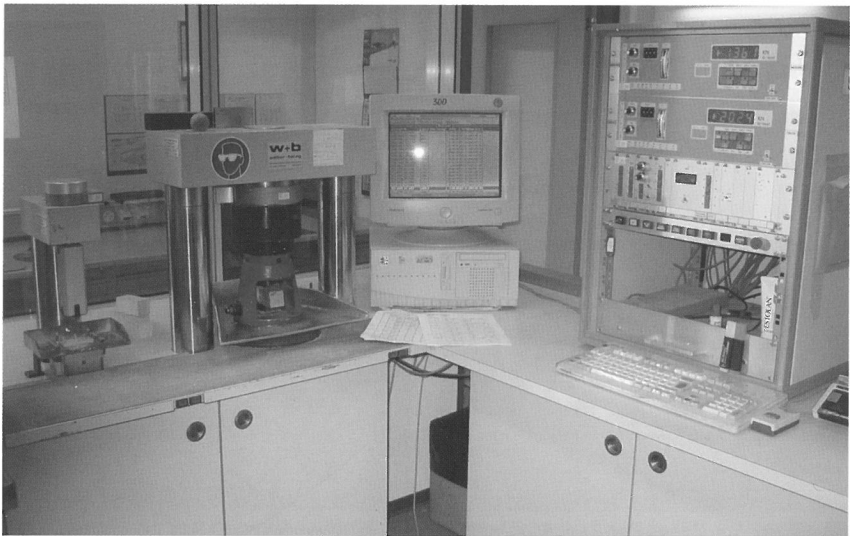
Fig. 37: core compression testing
