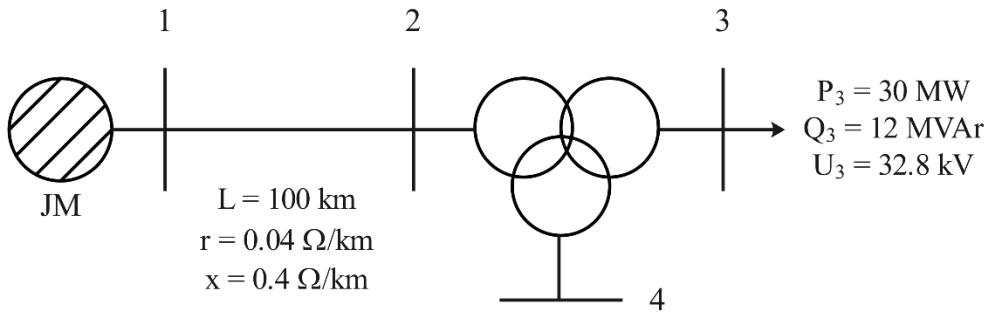
$$S_{1n} = 40 \text{ MVA}, S_{2n} = 40 \text{ MVA}, S_{3n} = 15 \text{ MVA}$$
