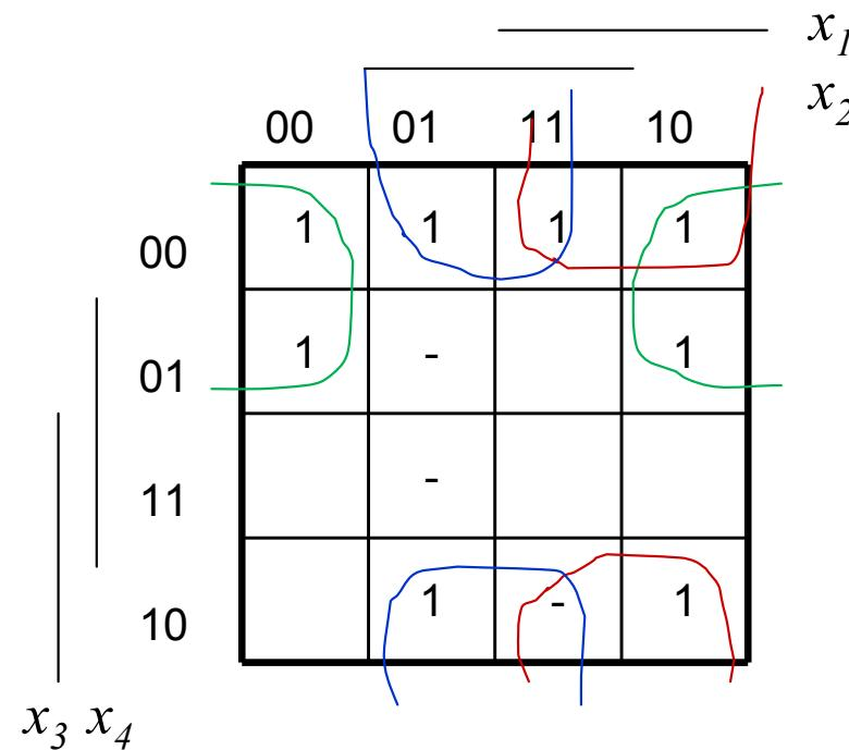
$$F = \sum(0, 1, 4, 6, 8, 9, 10, 12) + d(5, 7, 14) = \overline{\overline{x_2}}\overline{x_3} + \overline{x_1}\overline{x_4} + \overline{x_1}\overline{x_2}$$
