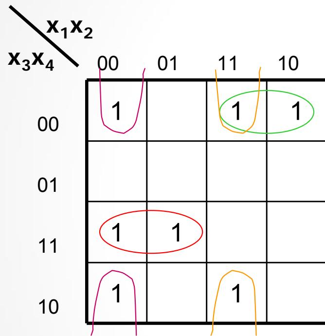
$$y_{\min} = \bar{x}_1 \bar{x}_2 \bar{x}_4 + \bar{x}_2 \bar{x}_3 \bar{x}_4 + \bar{x}_1 x_3 x_4 + x_1 x_2 \bar{x}_4$$
