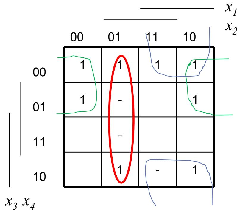
$$F = \sum(0, 1, 4, 6, 8, 9, 10, 12) + d(5, 7, 14) = \overline{x_2} \overline{x_3} + x_1 \overline{x_4} + \overline{x_2} \overline{x_4}$$
