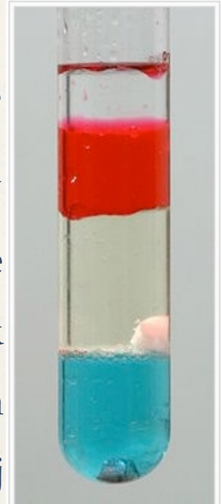
A density column containing some common liquids and solids. From top: baby oil, rubbing alcohol, vegetable oil, wax, water, and aluminum. Food coloring was added to rubbing alcohol and water for visibility.
