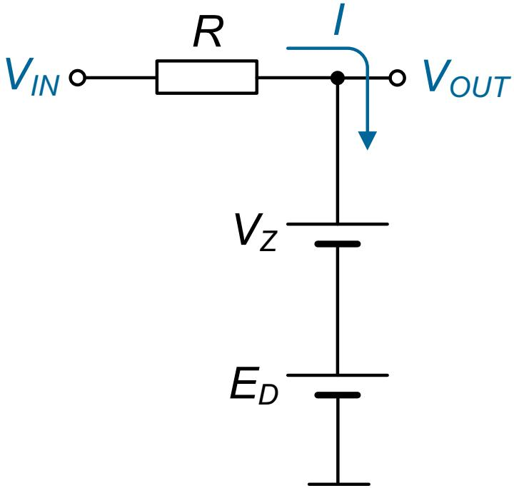
$$V_{OUT} = E_D + V_Z = 4 \text{ V}$$
