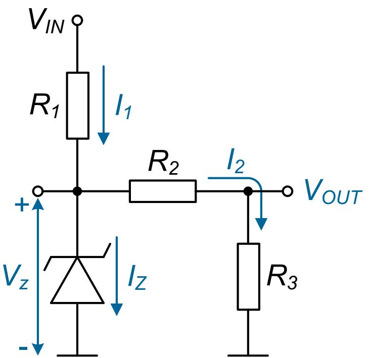
$$V_{OUT} = \frac{R_3}{R_2 + R_3} V_Z \Rightarrow R_2 = R_3 \left( \frac{V_Z}{V_{OUT}} - 1 \right)$$
