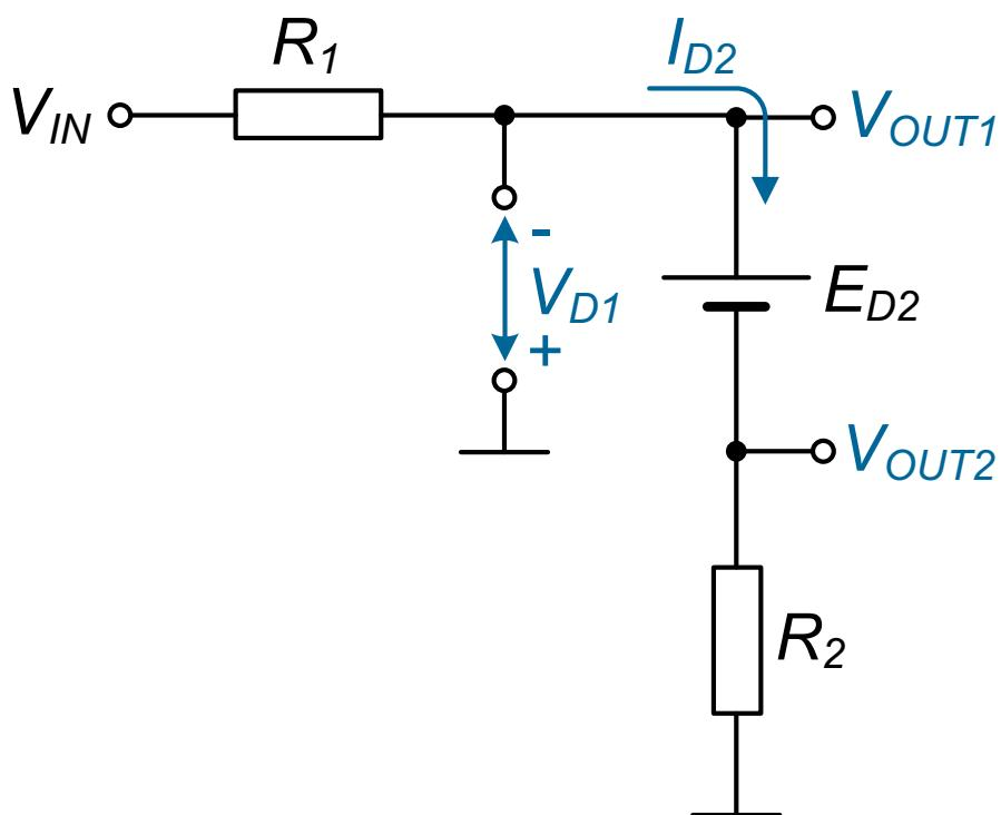
$$I_{D2} = \frac{V_{IN} - E_{D2}}{R_1 + R_2} > 0 \text{ A}$$
