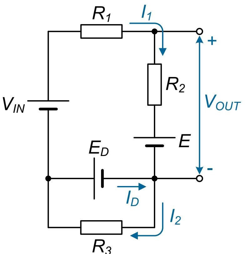
$$I_1 = \frac{V_{IN} - E + E_D}{R_1 + R_2} = -165 \mu\text{A}$$
