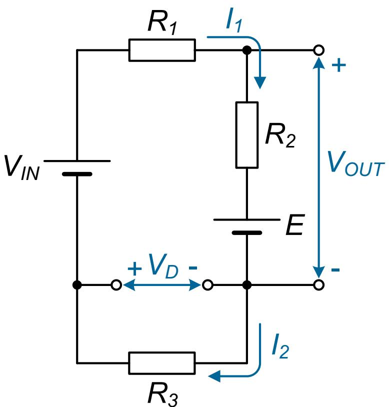
$$I_1 = I_2 = \frac{V_{IN} - E}{R_1 + R_2 + R_3} = 116.67 \mu\text{A}$$
