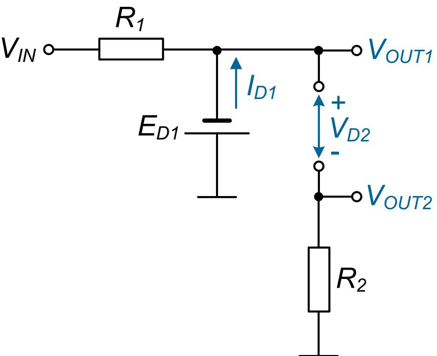
$$I_{D1} = \frac{-E_{D1} - V_{IN}}{R_1} > 0 \text{ A} \Rightarrow V_{IN} < -E_{D1}$$
