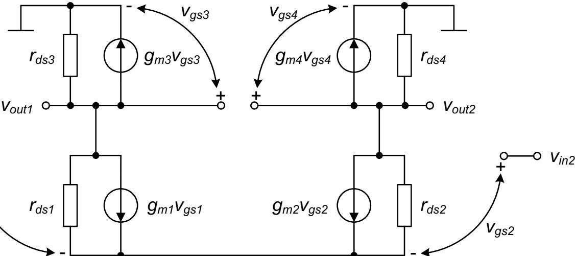
$$v_{gs3} = v_{out1}$$
