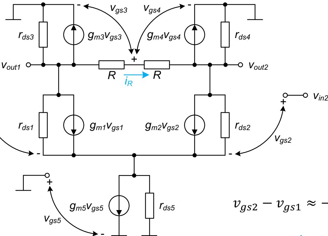
$$v_{in1} - v_{gs1} + v_{gs2} - v_{in2} = 0$$
