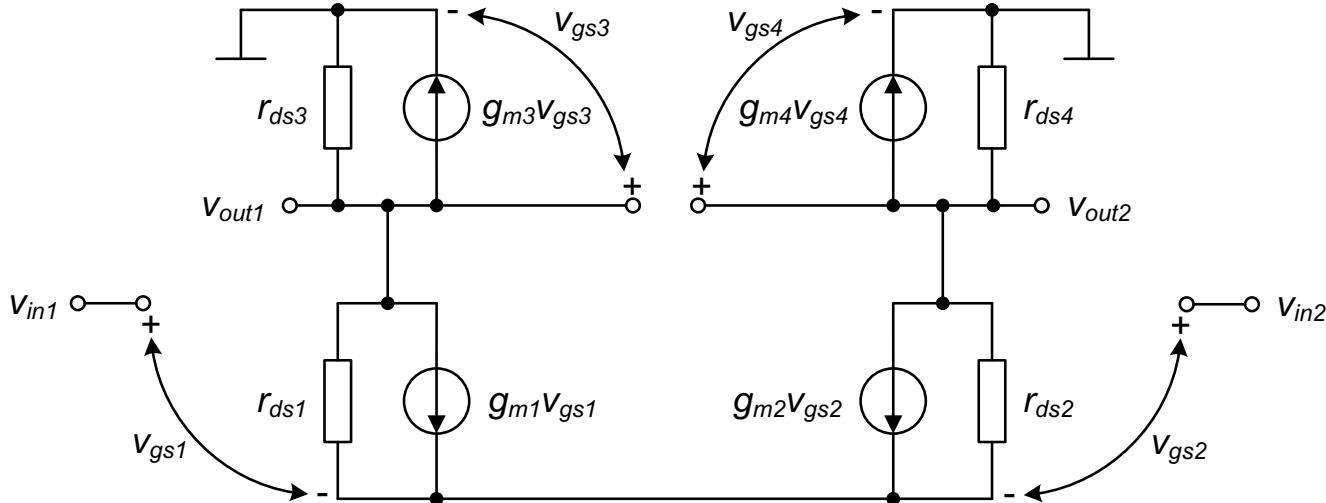
$$g_{m1}(v_{gs1} + v_{gs2}) + \frac{v_{out1} + v_{out2}}{r_{ds1}} - \frac{v_{in1} + v_{in2}}{r_{ds1}} = 0$$
