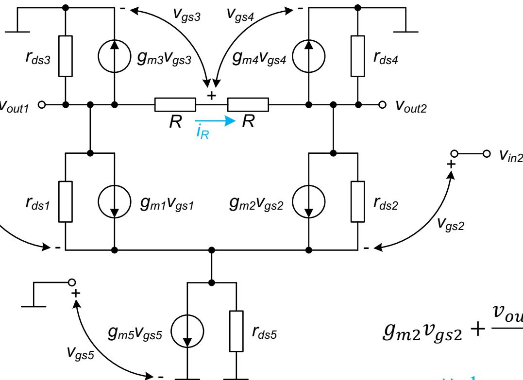
$$i_R = \frac{v_{out1} - v_{gs3}}{R} = \frac{v_{gs4} - v_{out2}}{R}$$
