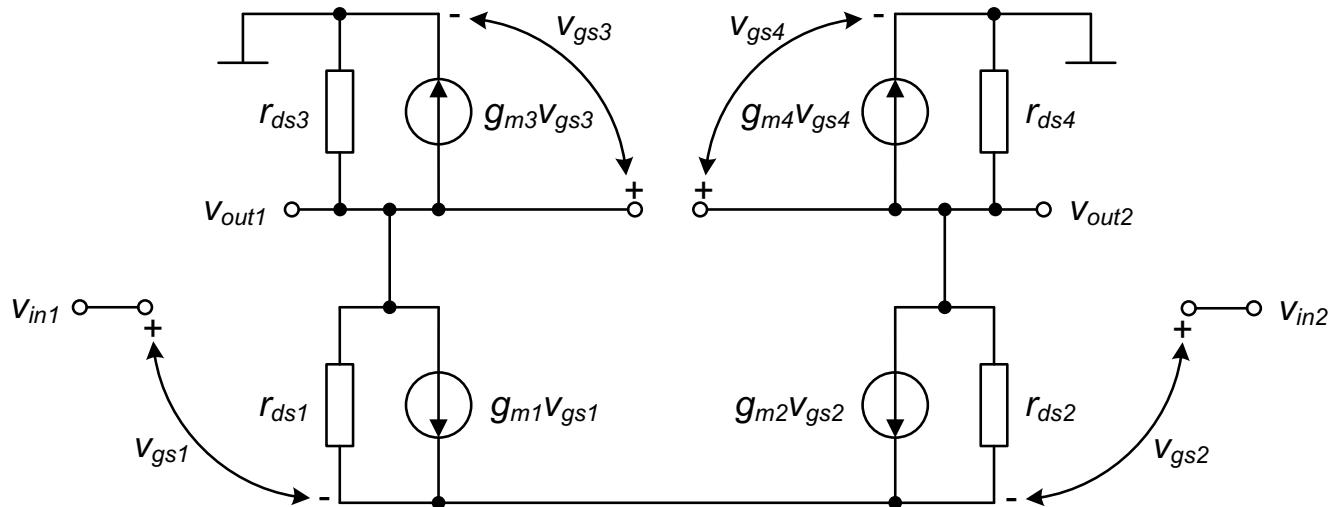
$$g_{m1}v_{gs1} + \frac{v_{out1} + v_{gs1} - v_{in1}}{r_{ds1}} + g_{m2}v_{gs2} + \frac{v_{out2} + v_{gs2} - v_{in2}}{r_{ds2}} = 0$$
