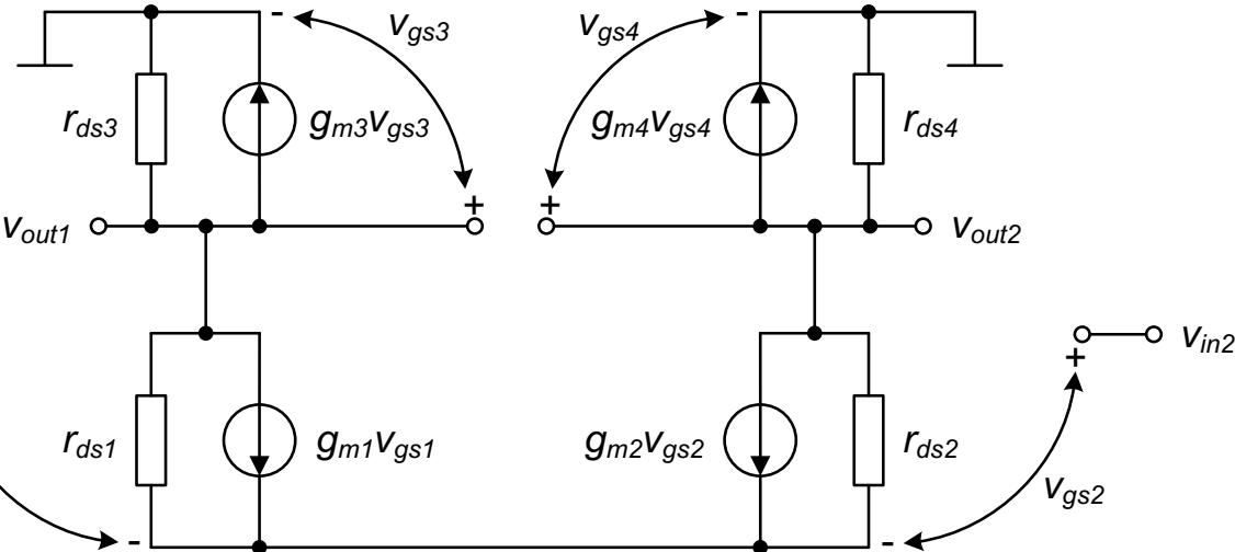
$$v_{in1} - v_{gs1} + v_{gs2} - v_{in2} = 0$$
