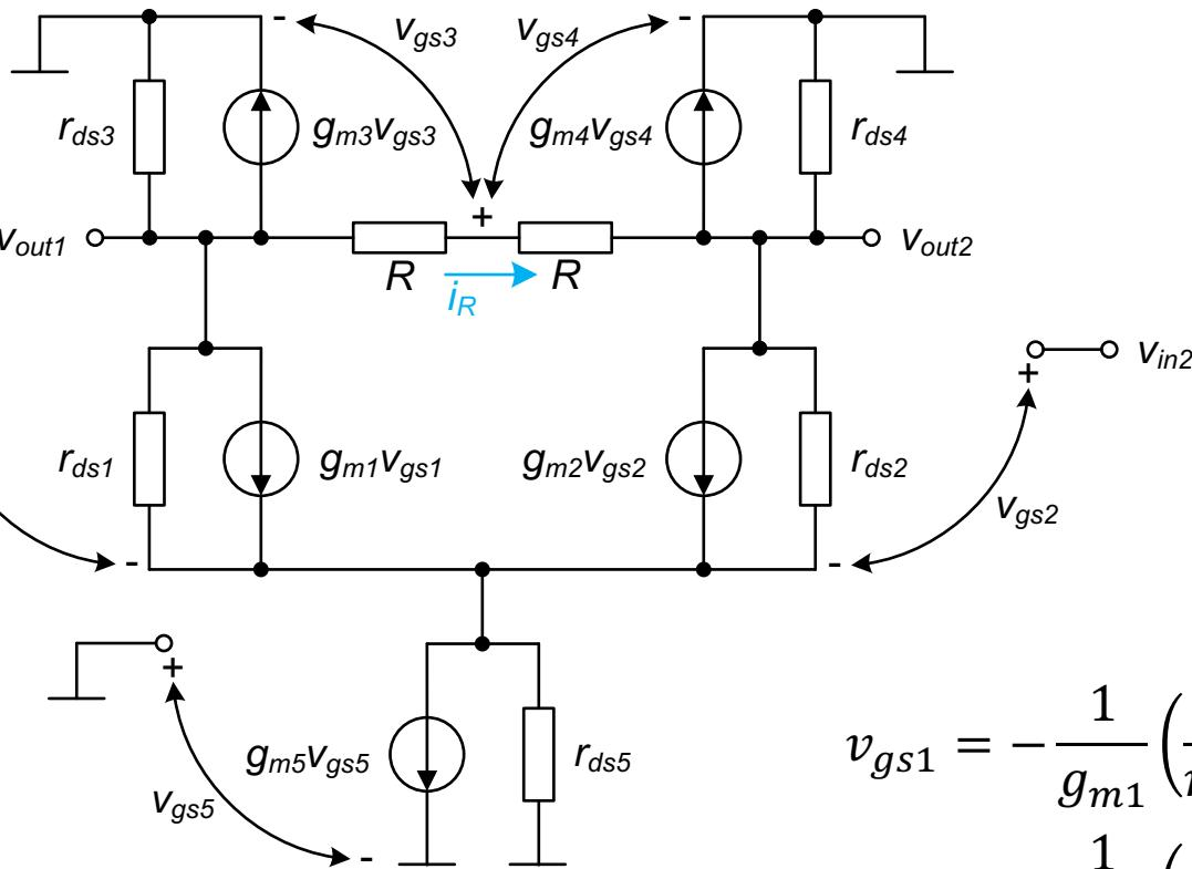
$$v_{in1} - v_{gs1} + v_{gs2} - v_{in2} = 0$$
