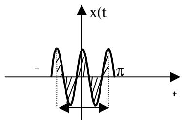
$$\int_{-\pi}^{\pi} \cos(2t) dt = 0 \quad \int_{-\pi}^{\pi} \cos(nt) dt = 0 \quad \text{Osim ako je } n=0, \text{ kada je } \int_{-\pi}^{\pi} 1 \cdot dt = 2\pi.$$
