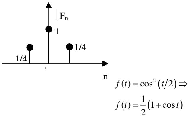
$$F_n = \frac{1}{2\pi} \int_{-\pi}^{\pi} f(t) e^{-jnt} dt = \frac{1}{2\pi} \int_{-\pi}^{\pi} \left( \frac{1}{2} + \frac{1}{4}e^{jt} + \frac{1}{4}e^{-jt} \right) e^{-jnt} dt$$
