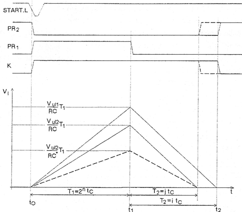
$$V_I(t_1) = \frac{1}{RC} \cdot \int_{t_0}^{t_1} V_{ul} dt$$
