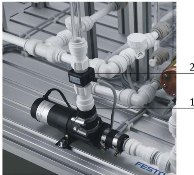
Controlled flow rate system – pump P101 with flow sensor B102 (measuring point FIC 101)
