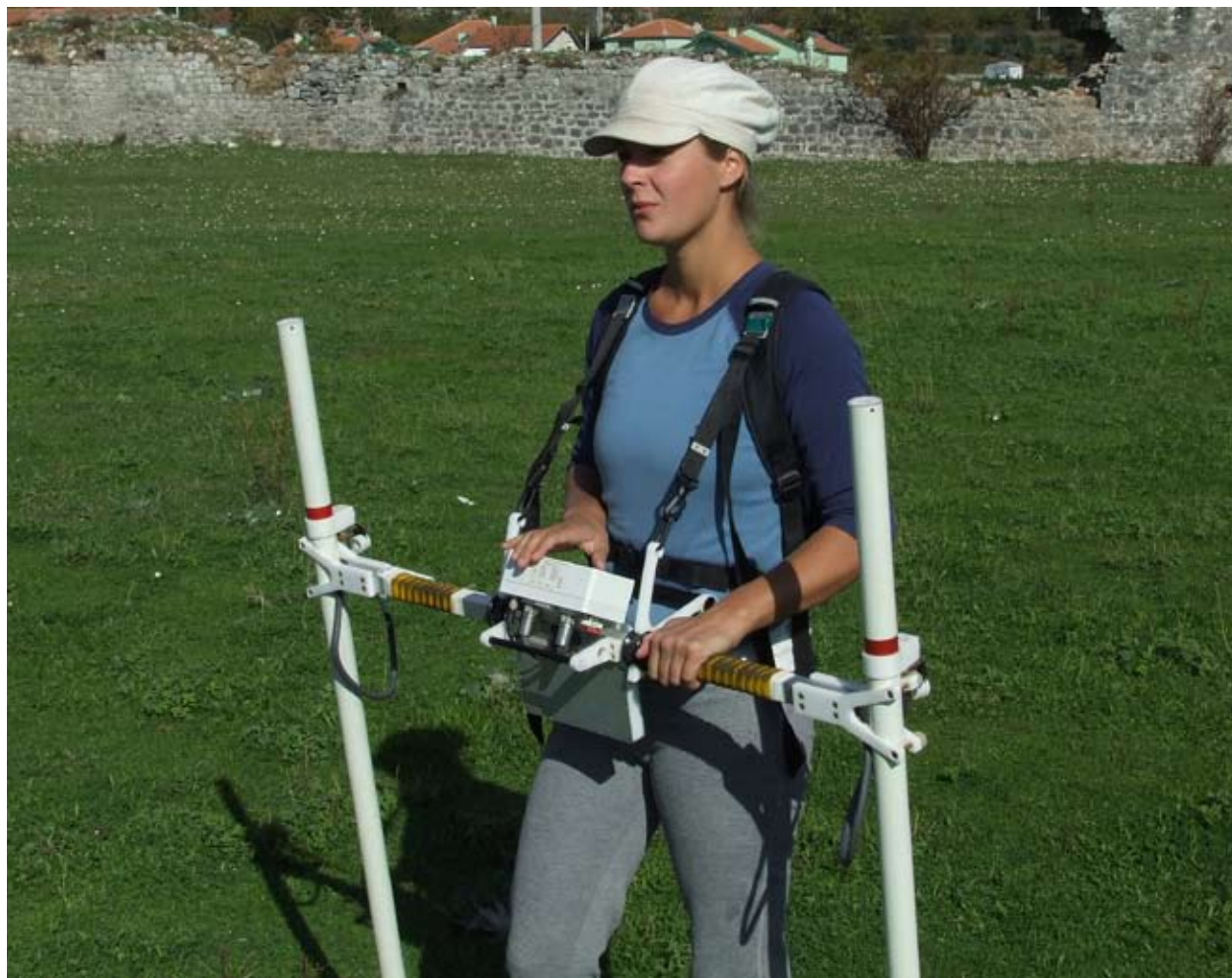
Plate. 3 : Bartington Grad 601-2 with operator (photo: S.Hay)
