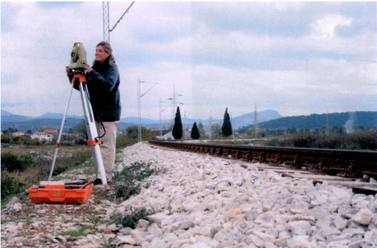
Plate. 2: Setting out the grid using a Total Station (photo: L.Pett)
