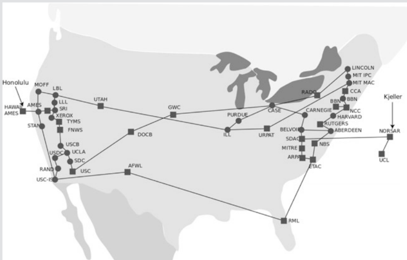
■ Fig. 2.2 The ARPANET in 1974. Note that the first node outside the US was at Kjeller in Norway. (Public domain, source: ► https://commons.wikimedia.org/wiki/File:Arpanet_1974.svg )
