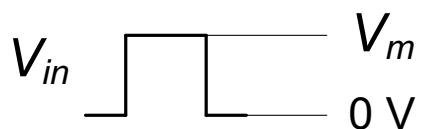
$$C \frac{dv_c(t)}{dt} = \frac{V_{in} - v_c(t)}{R}$$
