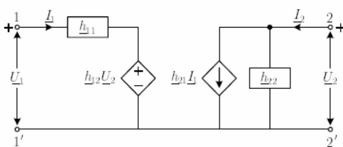
$$\underline{U}_1 = h_{11} \underline{I}_1 + h_{12} \underline{U}_2$$
